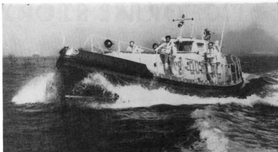
The steel-hulled 48-foot 6-inch Oakley Mark III life-boat which is now at Ross-lare Harbour, County Wexford. The R.N.L.I. is fully satisfied that steel hulls are in every way as satisfactory as wooden hulls, and at present nine steel life-boats of other classes are in service in the Institution's fleet.
