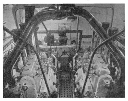
THE ENGINE-ROOM. The two 40-h.p. Diesel engines on board the Violet Armstrong, the 46-feet Watson cabin motor life-boat, stationed at Appledore, North Devon, in 1938. The big black pipes are the exhausts running up to the funnel.
