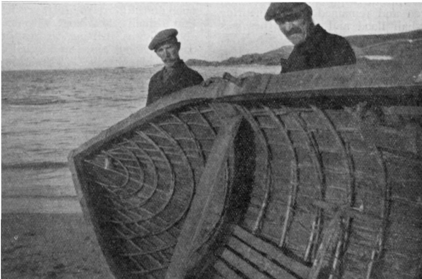
The inside of the curragh, showing its ribs of hazel stick, with the bark still on, tied together with string and bits of line, and covered with calico and tar. Mr. McFadden and Mr. Carr both received the Institution's thanks on vellum for their gallantry. (See " The Life-boat " for June, 1932.)
