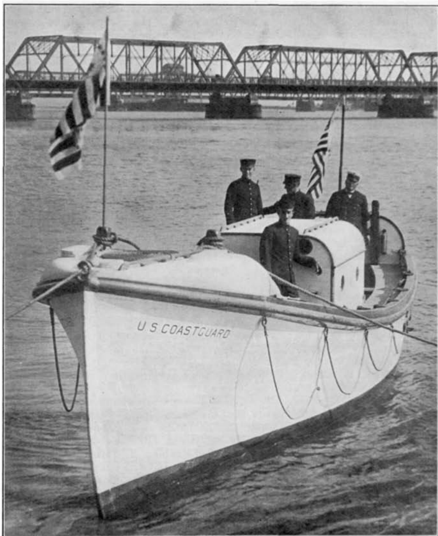
36-FOOT MOTOR SELF-BAILING, SELF-RIGHTING LIFE-BOAT, U.S. COAST GUARD.
